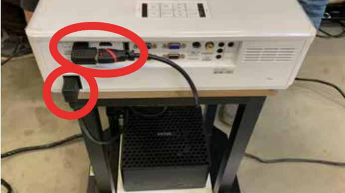
3.1 Each beamer needs a power cable and a video cable connected
