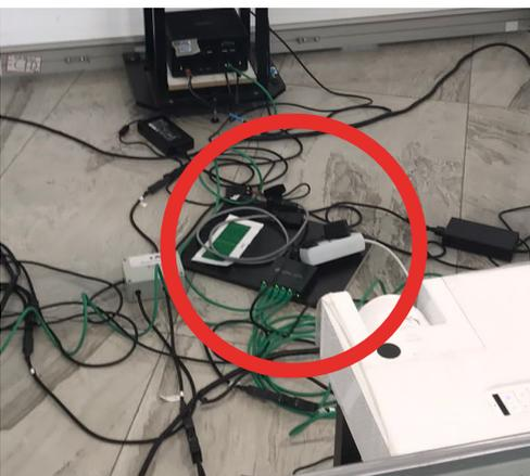
3.5 Connect a short green network cable (CAT 6A) to each of the computers. Connect the four cables to the TP Switch on the wooden plate. Also, connect the long green network cable (CAT 6A) to the TP Switch on the wooden plate and pull it outside the frame. Connect the white box and the TP Switch on the wooden plate to a white multiple plug. Pull the cable of the multiple plug outside the frame.
