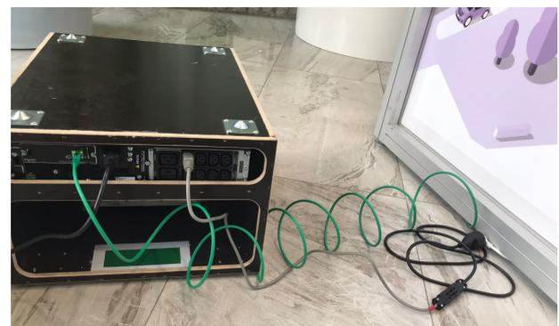
3.6 Connect the long green network cable to the UPS. Also, connect the cable of the multiple plug to the UPS (use adapter cable provided). Connect the UPS to the socket.
